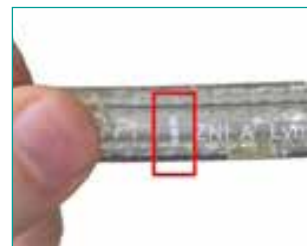
2. Cut rope light neatly
