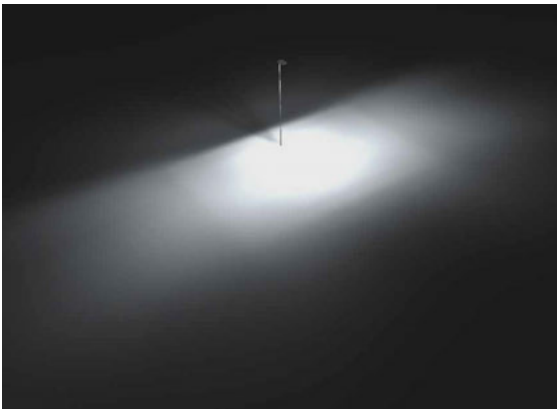
Asymmetric Optic Front 40° - Side 60° Asymmetric distribution with medium bilateral emission.
