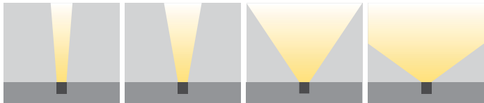
XN: Extra Narrow Angle N: Narrow Angle W: Wide angle XW: Without lens
