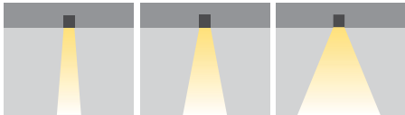
XN: Extra Narrow Angle N: Narrow Angle M: Medium Angle
