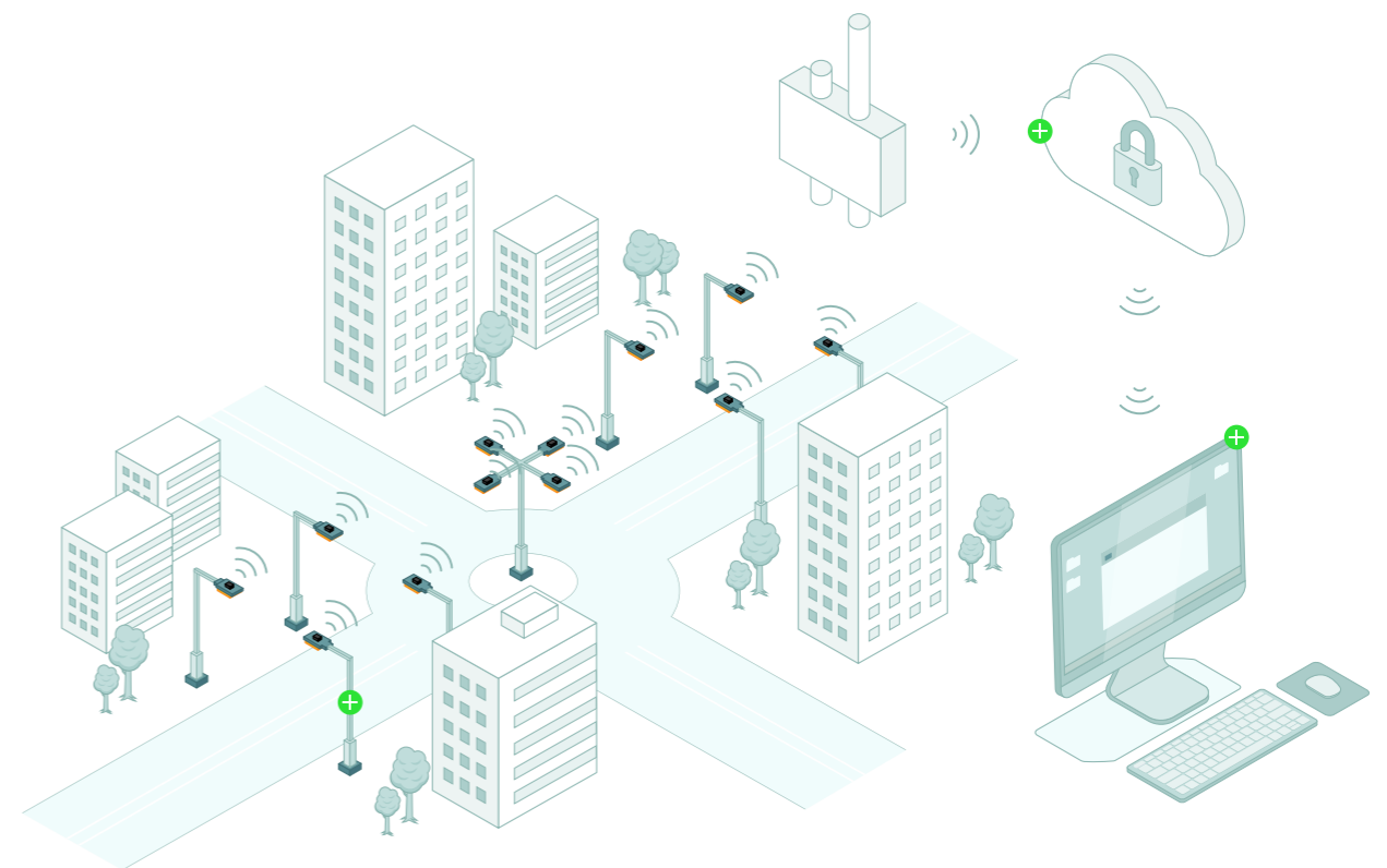
CLUE CITY operating diagram. Two-way communication and lighting management.
