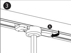
Rotate tab (A) clockwise 90° to connect the adaptor to the neutral circuit.
