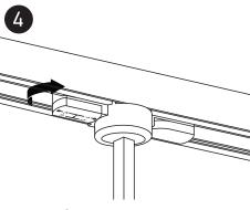
Rotate tab (3) to the desired position circuit.
