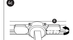
Circuit 2: To connect to circuit 2, from the starting position, rotate the tab **(B)** anti-clockwise 90°.
