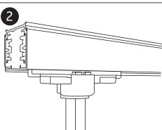
Ensure the track adaptor is inserted with the correct orientation.
