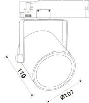
COB 3000 [K] STANDARD Light colour CRI 2445 [lm] Led chip flux Luminous flux 2200 [lm] System power 19 [W] Luminaire Efficiency 116 [lm/W] Beam angle 38° Controller ON/OFF MacAdam 3 SDCM
