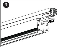
Rotate adaptor lock **B** clockwise 90° to connect the adaptor to the neutral circuit.
