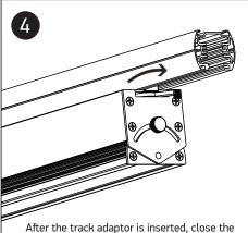
After the track adaptor is inserted, close the security button on the adaptor.
