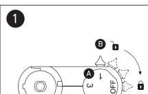
To mount the track adaptor into the track system, first check that the selector knob  $oldsymbol{\mathbb{A}}$  is at OFF position and the adaptor lock **B** is disengaged.
