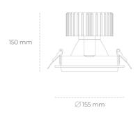
COB 3000 [K] HI EFFICIENT Light colour CRI 90 Led chip flux 5801 [lm] Luminous flux 4640 [lm] System power 36 [W] Luminaire Efficiency 129 [lm/W] Beam angle 60° Controller ON/OFF MacAdam 3 SDCM
