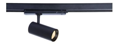
The Driver of this dimmable Trackspot is located in the Trackadaptor, so the heat from both the LEDs and the Driver can be dissipated separately. This ensures good heat dissipation and a longer lifespan.
