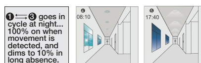
1. DISP goes in cycle at night... 100% on when movement is detected, and dims to 10% in long absence. When the natural light level exceeds setpoint of the light, the light will turn off even if the space is occupied. The light automatically turns on at 10% when natural light is insufficient (no motion).
