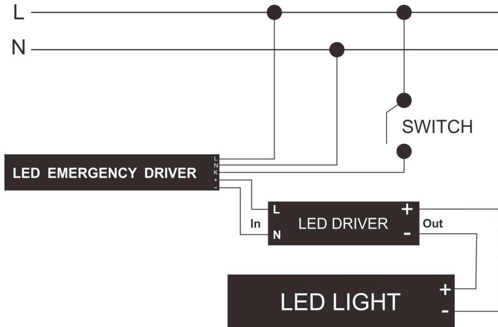
**Warning: the switch wire must be in the same phase with charging wire!**
